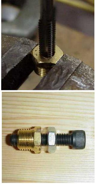
**4.** Take the jam nut and thread it part way up the Bolt. Wrap the Bolt with Teflon tape, to prevent air leaking between the threads, and thread the Bolt and nut into the Cap, place aside for now. I will refer to this as the 'Cap Assembly'.
